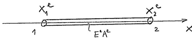
$$\bullet \underline{N}^e = \frac{1}{L^e} \begin{bmatrix} x_2^e - x & x - x_1^e \end{bmatrix} \rightarrow \underline{B}^e = \frac{d}{dx} \underline{N}^e = \frac{1}{L^e} \begin{bmatrix} -1 & 1 \end{bmatrix}$$
