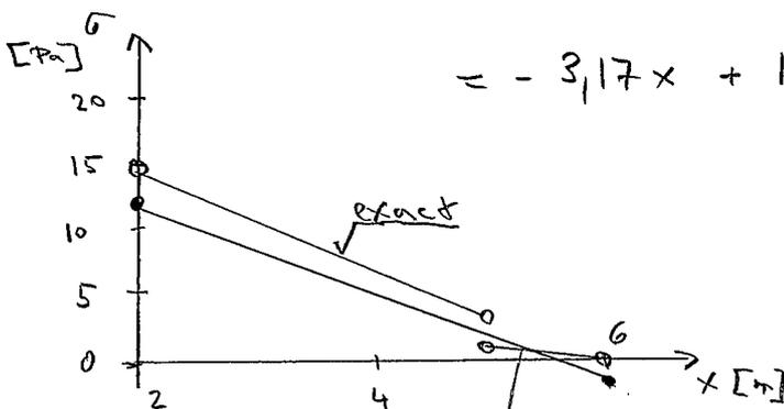
FEM - no. jump  $\Rightarrow$  node should be always placed where a point force is applied
