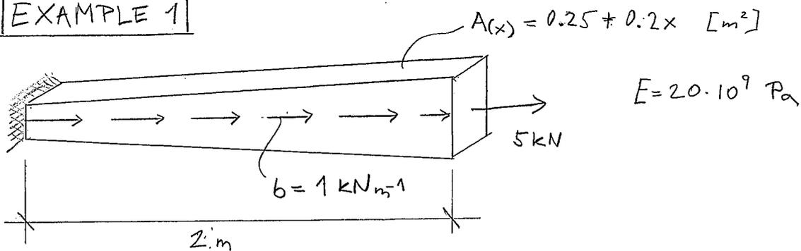
→ 2 nodes, 1 element, with linear basis functions
