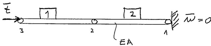
$$\text{weak solution: } \int_0^L \left( \frac{dw}{dx} \right)^T EA \left( \frac{dw}{dx} \right) dx - \int_0^L (\underline{Jw})^T \bar{b} dx - \left[ (\underline{Jw})^T \bar{F} A \right]_{x=0} = 0$$
