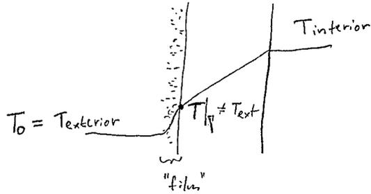
$$Q|_{\Gamma} = \alpha(x) (T_{\Gamma} - T_0)$$
