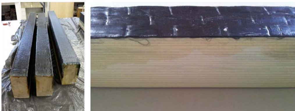
Fig. 6 Glulam beam reinforced by a carbon fiber sheet [2]
