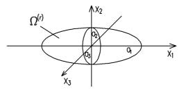
Fig. 3.1: Ellipsoidal inclusion in an unbounded domain
