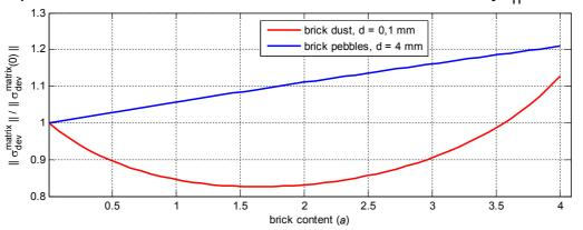
dependence of deviatoric stress in matrix on crushed brick content loaded by  $\sigma_{11} \neq 0$  and  $\sigma_{12} \neq 0$
