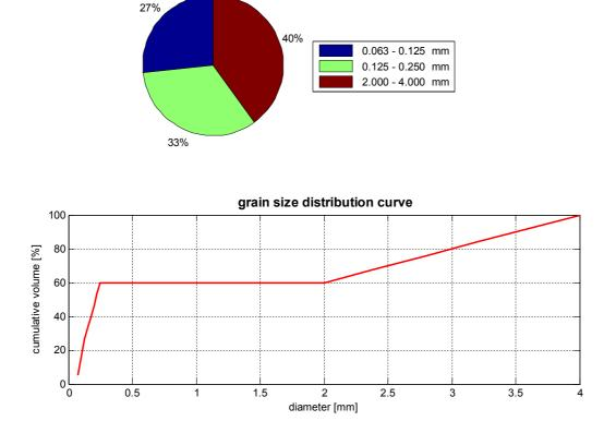
Fig. 9.6: Modified crushed brick size distribution
