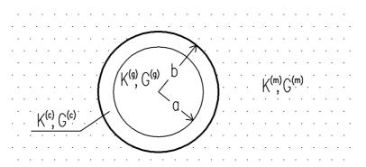
Fig. 5.1: A three-phase composite spherically concentric solid
