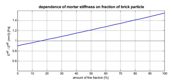
Fig. 9.4: Dependence of mortar stiffness on diameter of brick particles
