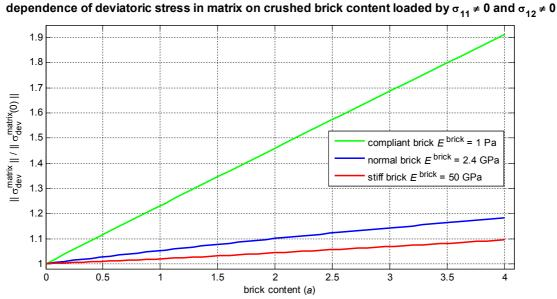
Fig. 7.5: Dependence of quadratic average of deviatoric stress in mortar on content of crushed bricks for different brick stiffness
