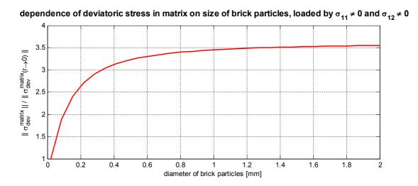
Fig. 9.2: Dependence of deviatoric stress increase in matrix on diameter of brick particles
