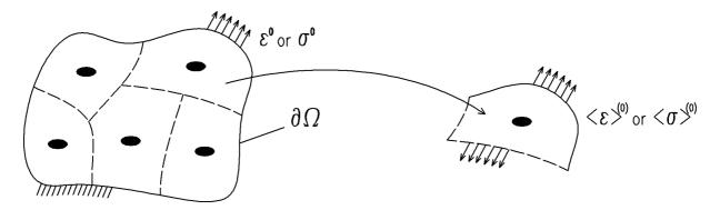
Fig. 3.4: Interaction of inhomogeneities in the Mori-Tanaka model [4]
