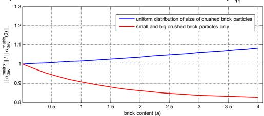
dependence of deviatoric stress in matrix on crushed brick content loaded by  $\sigma_{11} \neq 0$  and  $\sigma_{12} \neq 0$
