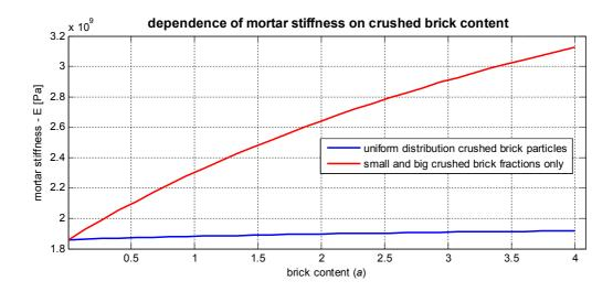
Fig. 9.7: Dependence of mortar stiffness on brick content
