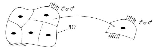
Fig. 3.3: Model of dilute phase distribution [4]
