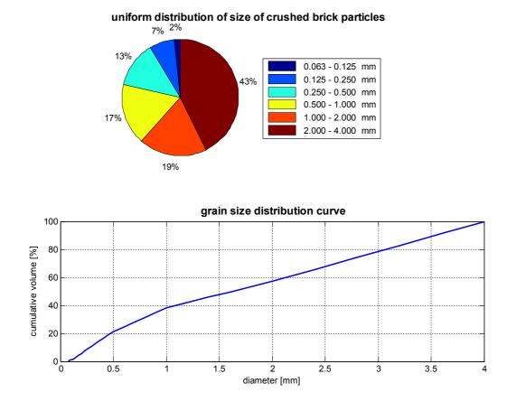
Fig. 9.5: Approximate distribution of crushed brick size in ancient Byzantine structure
