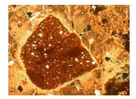
Fig. 6.2: Fragment of pottery in cocciopesto with thin layer of C-S-H [15]
