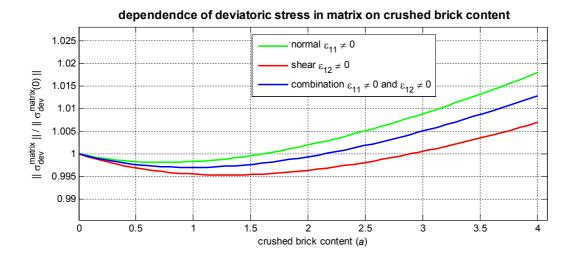
Fig. 7.4: Dependence of quadratic average of deviatoric stress in mortar on content of crushed bricks
