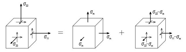
Fig. 2.1: Decomposition of stress in hydrostatic and deviatoric part
