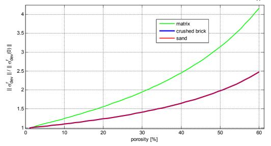
dependence of deviatoric stress in individual phases on crushed brick content if loaded by  $\sigma_{11} \neq 0$  and  $\sigma_{12}$
