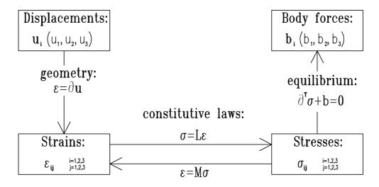
Fig. 1.1: Diagram of kinematic and static equations
