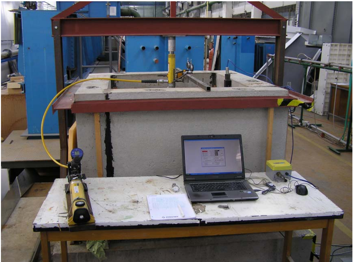
Fig. 25. Fully equipped stand for plate load test with shear zone and lateral pressure measurement
