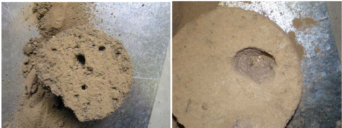
Fig. 42. Internal erosion experiments - cut through specimens after collapse
