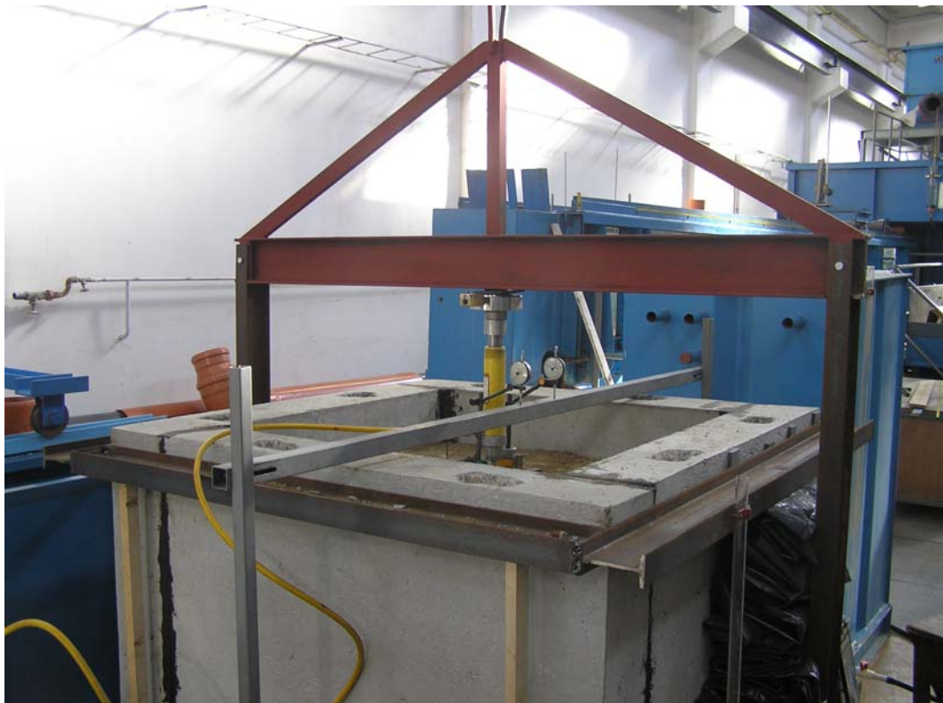
Fig. 12. Full scale plate load test on the soil specimen
