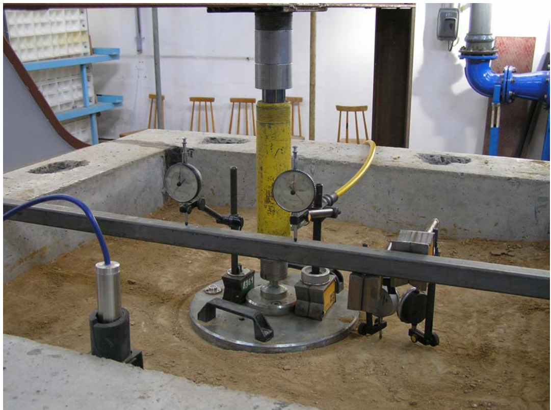
Fig. 26. Detail view on the analogue settlement measuring devices (later on digital)
