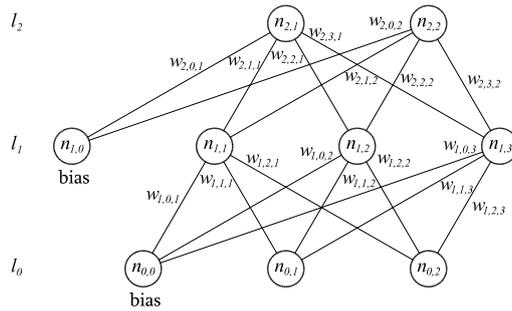
Figure 1: Architecture of multi-layer perceptron
