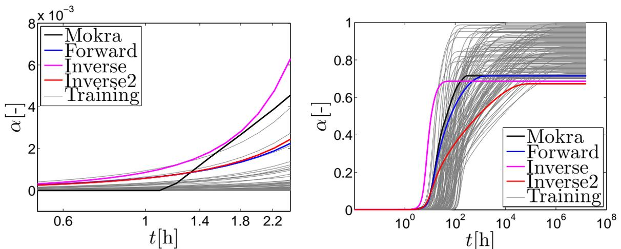
Figure 5: Comparison of experimentally obtained degree of hydration for “Mokra” cement with simulations for model parameters identified using prepared ANNs.
