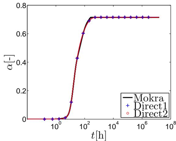
Figure 4: Comparison of experimentally obtained degree of hydration for “Mokra” cement with simulations for directly optimised model parameters.
