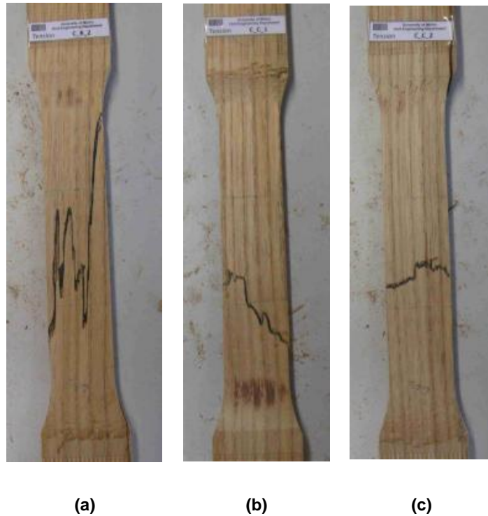
Figure 136 – Examples of tension specimens failed in split (a), shear (b) and tension (c)
