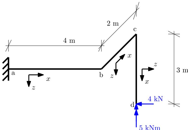
Kontrola.  $N^{ba} = -4$  kN,  $M_x^{bc} = +12$  kNm,  $V_z^{cd} = -4$  kN,  $M_y^{cd} = 12$  kNm,  $M_y^{ba} = -12$  kNm,  $V_y^{bc} = -4$  kN,  $M_z^b = -13$  kNm,  $M_z^{cb} = -5$  kNm.
