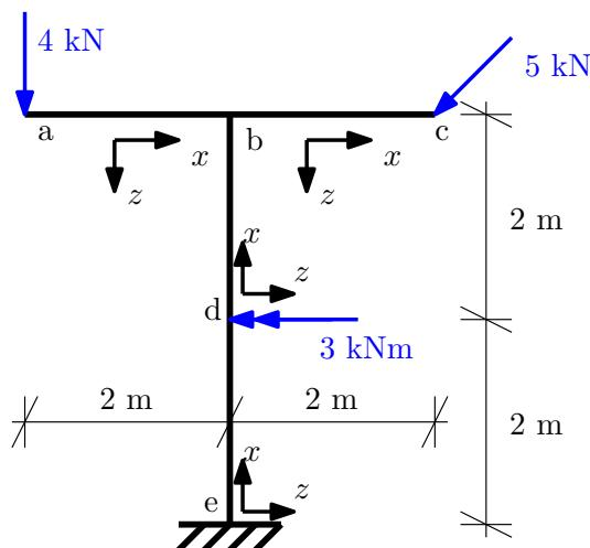
Kontrola.  $N^{bd} = -4$  kN,  $M_x^{bd} = -10$  kNm,  $V_z^{ba} = -4$  kN,  $M_y^{ba} = -8$  kNm,  $M_y^{bd} = 8$  kNm,  $V_y^{bc} = 5$  kN,  $V_y^{bd} = 5$  kN,  $M_z^{bc} = 10$  kNm,  $M_z^e = 17$  kNm.
