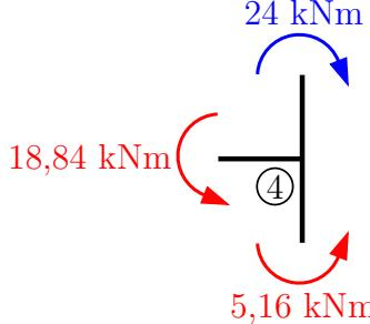
The diagram shows a vertical beam segment with a horizontal cut at node 4. Three clockwise moments are applied at this node: a blue moment of 24 kNm at the top, a red moment of 18,84 kNm on the left, and a red moment of 5,16 kNm at the bottom.
