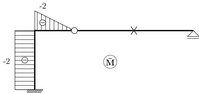
$$\bar{1} \cdot w_c = \int_{\ell} \frac{M \cdot \bar{M}}{EI_y} dx = \frac{1}{EI_y} \cdot \left\{ \begin{array}{c} M_y \\ \bar{M}_y \end{array} \right|_{-0,395}^{0,790} + \frac{1}{EI_y} \cdot \left\{ \begin{array}{c} M_y \\ \bar{M}_y \end{array} \right|_{-2}^2 \quad (1)$$
