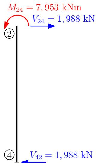
$$\textcircled{4} : 7,953 - V_{24} \cdot 4 = 0 \\ V_{24} = 1,988 \text{ kN}$$
