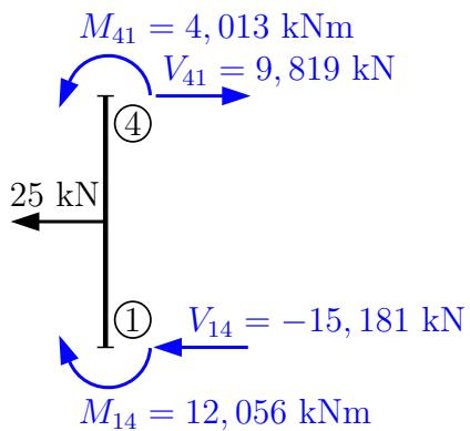
$$\textcircled{1} : \quad 4,013 - 12,056 + 25 \cdot 1,5 - V_{41} \cdot 3 = 0 \\ \mathbf{V}_{41} = 9,819 \text{ kN}$$
