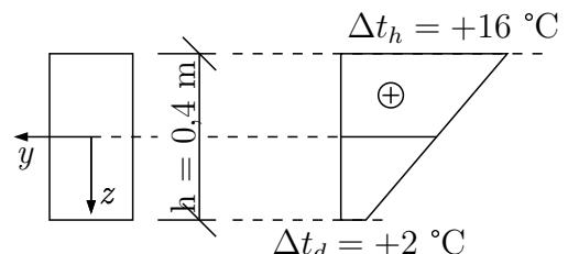
$$\Delta t_s = \frac{\Delta t_d + \Delta t_h}{2} = \frac{2 + 16}{2} = 9 \text{ °C}$$
