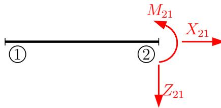
$$\begin{aligned} L_{21} &= 4 \text{ m} \\ k_{21} &= \frac{2 \cdot 20000}{L_{21}} = 10000 \text{ kNm} \\ n_{21} &= \frac{100000}{L_{21}} = 25000 \text{ kNm}^{-1} \end{aligned}$$
