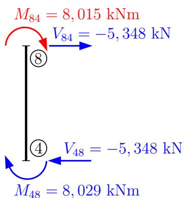
$$\textcircled{4} : \quad -8,015 - 8,029 - V_{84} \cdot 3 = 0 \\ \mathbf{V}_{84} = -5,348 \text{ kN}$$
