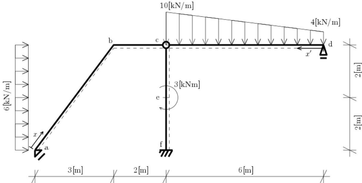
*Kontrola.*  $N^{ba} = -14,4$  kN,  $N^{cb} = -17,8$  kN,  $N^e = -19,36$  kN,  $V^{ab} = 7,74$  kN,  $V^{ba} = -11,46$  kN,  $V^e = 17,8$  kN,  $V^{cd} = 24$  kN,  $M^{ba} = -9,29$  kNm,  $M^f = -74,224$  kNm a maximální moment na intervalu a-b má velikost 7,8 kNm a na intervalu c-d má velikost 31,66 kNm.
