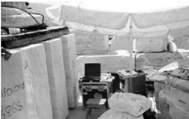
Fig. 7. Photograph of Dionysos marble blocks (seen to the left) together with the acoustic system. The test was performed on block number two from the front. The other blocks are original marble from the monument. Parts of the South wall are shown in the middle of the photograph.
