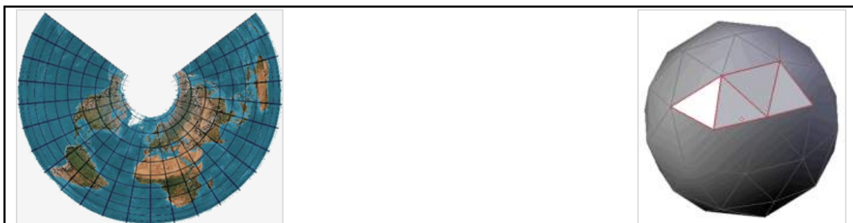
Figure 8-3: Double-curved surface in its projected (left) and discretized (right) shape Developing
