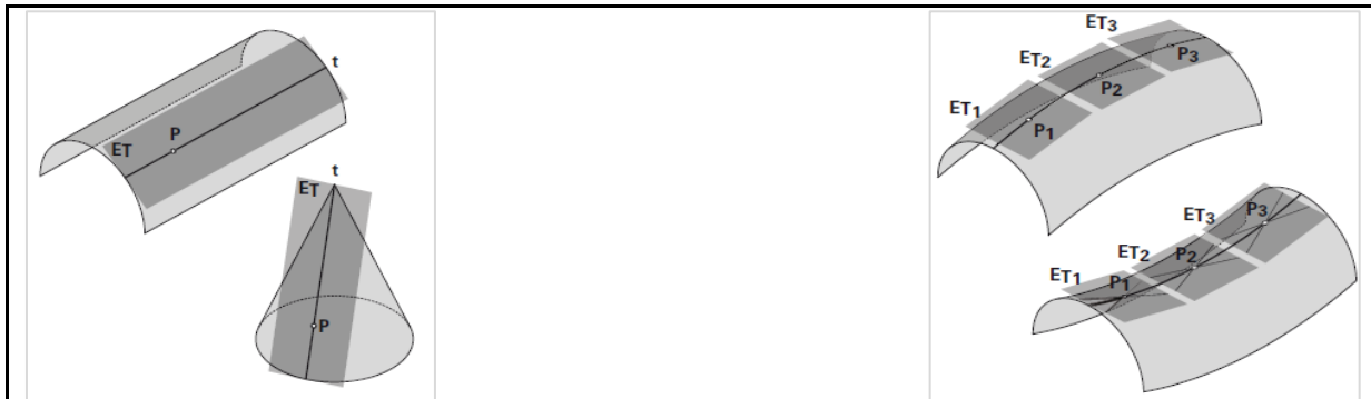
Figure 8-1: Single-curved (left) and double-curved (right) surfaces Dif. curvature ET = tangent plane; P=common point; t=tangent line
