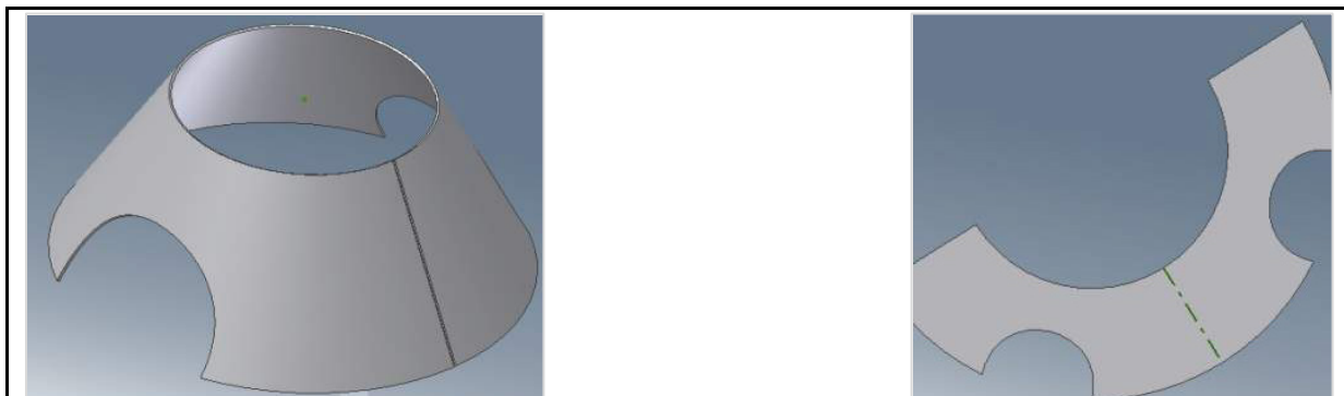
Figure 8-2: Single-curved surface (left) and its developed shape (right) Developing
