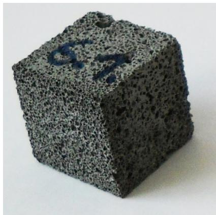
Figure 2: A typical fly ash foam specimen.
