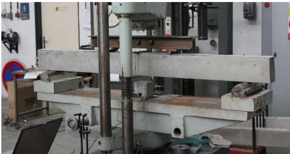
Figure 4.17: Test configuration of concrete beams
