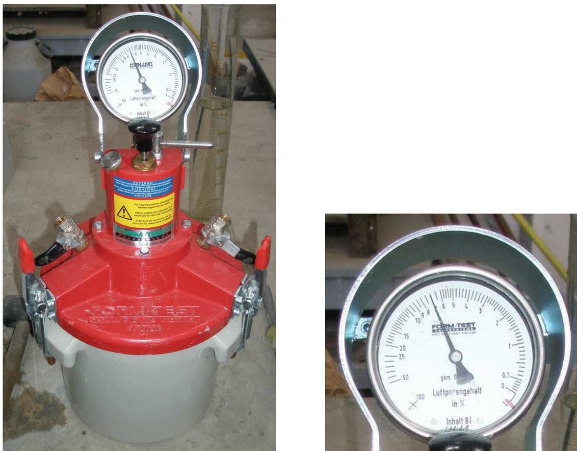
Figure 4.11: Air meter showing approximate air content
