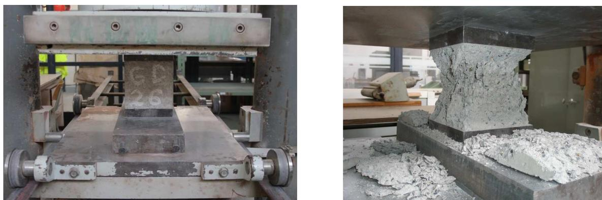
Figure 4.15: Test setup (left) and prescribed way of destruction of the sample (right)
