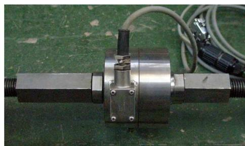
Figure 4.6: Close-up on load cell
