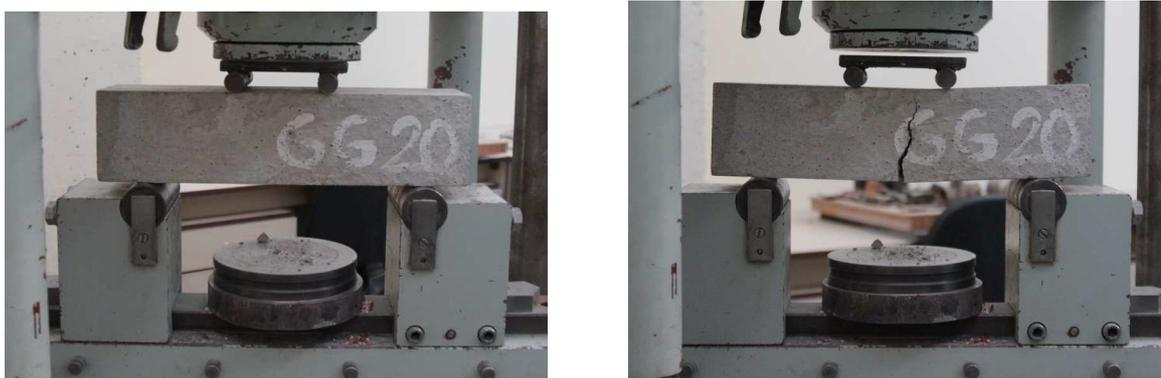
Figure 4.16: Test setup (left) and prescribed way of destruction of the sample (right)
