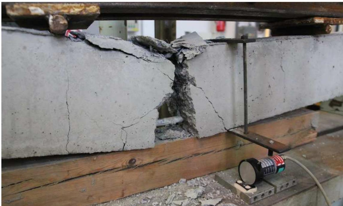
Figure 4.21: Collapsed beam by bending from group 2
