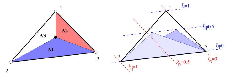
Equations  $\xi_i = const$  represents the set of lines parallel with the opposite edge of the *i*-th node. Equations corresponds to edges 2-3, 3-1, and 1-2 are  $\xi_1 = 0$ ,  $\xi_2 = 0$ , and  $\xi_3 = 0$ . The three nodes have coordinates (1,0,0), (0,1,0), and (0,0,1). Points in centers of edges have coordinates (1/2,1/2,0), (0,1/2,1/2), and (1/2,0,1/2), then the center of gravity (1/3,1/3,1/3).
