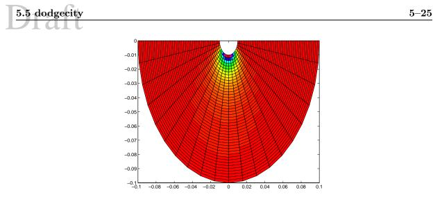
Figure 5.12: Stress plot for point Load on Semi-Infinite Domain
