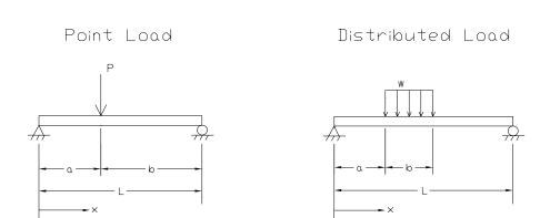
Figure 5.7: Simply Supported Beams with Various Loadings
