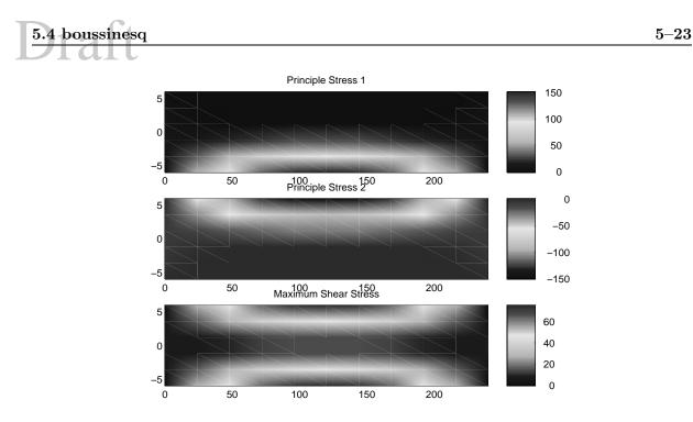
Figure 5.10: Sample output of principle stresses for *beam\_under\_load.m* with  $\omega = 2, b = 4, d = 12$ , and L = 20.
