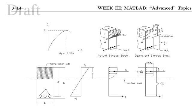
Figure 3.7: Equivalent and Exact Stress Distribution in Reinforced Concrete Beams
