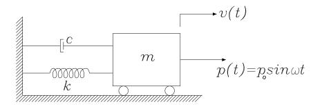
Figure 2.9: Single Degree of Freedom Oscillator
