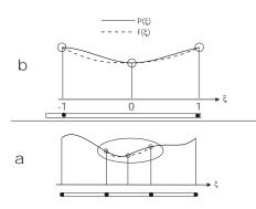
Figure 3.1: Newton-Cotes Numerical integration
