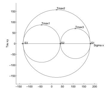
Figure 5.29: Example 3(c): Mohr's circle of 3-D stress.
