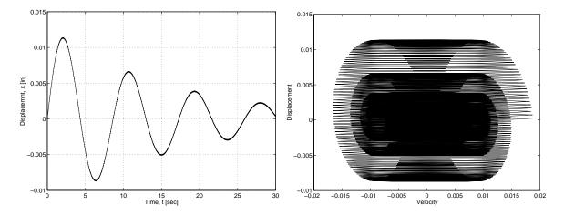
Figure 3.6: Runge-Kutta Solution for the Mass-Spring-Damper System
