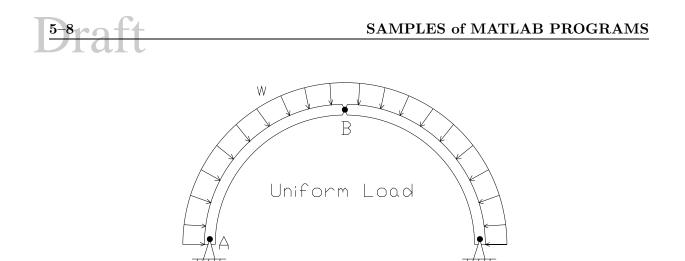
Figure 5.5: Simply Supported Arch with Uniform Load
