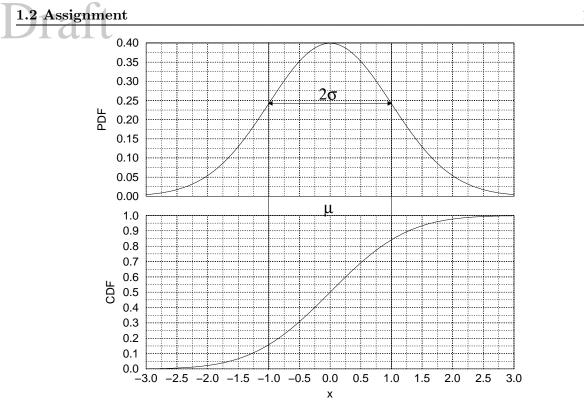
Figure 1.8: Normalized Gauss Distribution, and Cumulative Distribution Function
