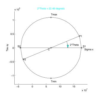
Figure 5.28: Example 2(e): Mohr's circle of 2-D stress.
