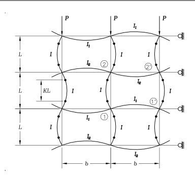
Figure 5.16: Column Effective Length in a Frame
