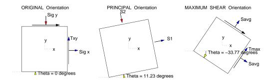
Figure 5.27: Example 2(b,d): Original, Principal and Maximum Shear Stresses.
