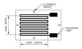
Figure 2.6: Bonded Strain Gage
