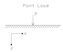
Figure 5.11: Point Load on Semi-Infinite Domain
