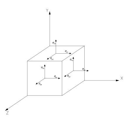
Figure 5.18: 3-Dimensional Stress Element
