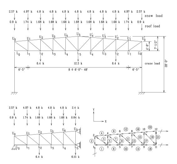
Figure 2.8: Steel Truss
