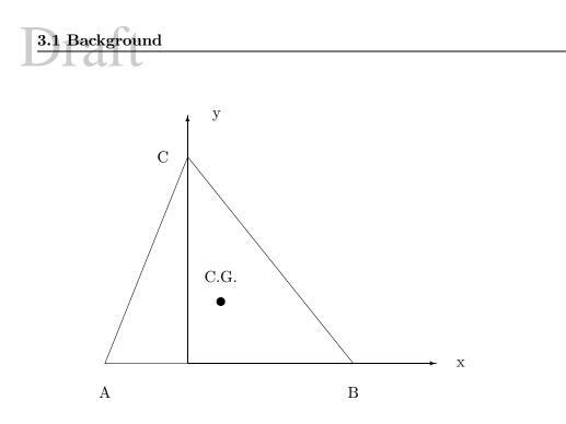
Figure 3.2: Center of Gravity and Moments of Inertia of A Triangular Cross-Section
