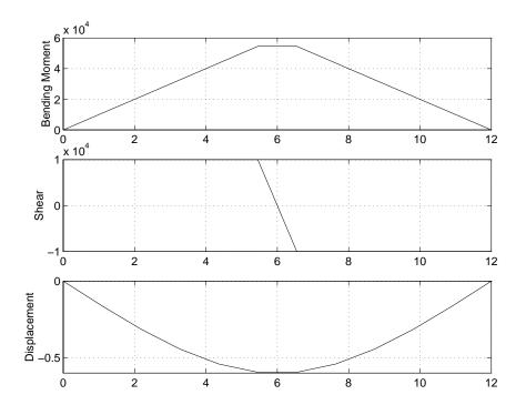
Figure 5.8: Sample output of BMdemo.m with a pointload using P = 20 kN, a = 6 m, L = 12 m, E = 200 GPa, I = 6e6 mm<sup>4</sup>, and 12 discretization points.
