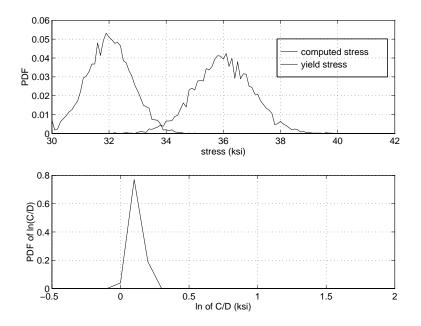
Figure 5.19: Sample output for a monte carlo simulation for a simply supported beam under a point load at the midspan.
