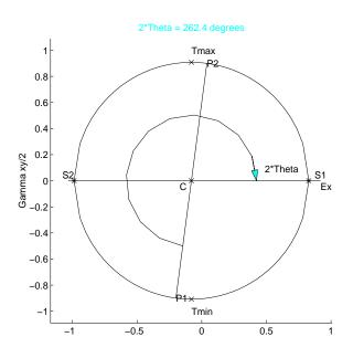
Figure 5.26: Example 1(d): Mohr's circle of 2-D stress.
