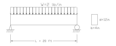
Figure 5.9: Beam Under Continuous Load
