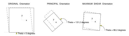
Figure 5.25: Example 1(c): Original, Principal, Maximum Shear Stresses, and Deformed shapes.
