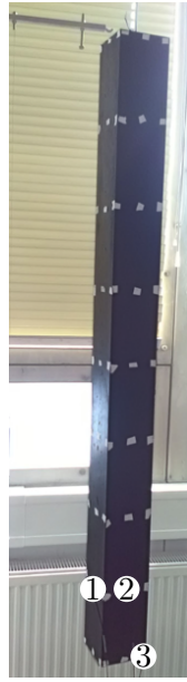
Figure 2.12: Free-free-vibration validation setup. Locations of 54 impact points are indicated by gray squares and positions of 3 accelerometers are marked by white circles.
