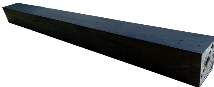
Figure 2.10: Manufactured prototype of a composite beam with optimized stiffening internal structure.
