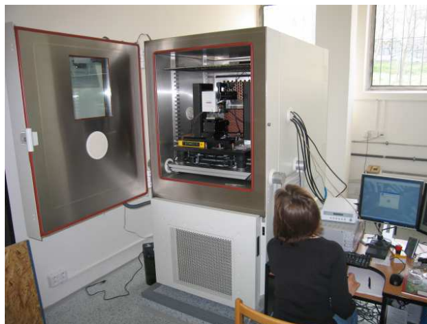
Figure 2: Nanoindentation - testing set-up
