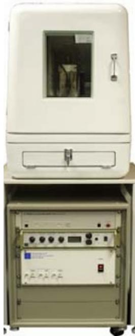
Figure 1.7: Hysitron Tribolab system.
