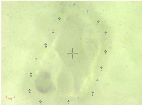
Figure 3.12: High-density C-S-H zone with prescribed indents as seen in optical microscope of CSM nanohardness tester.
