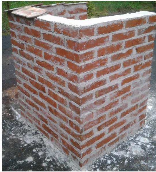
Figure 6.1: Masonry wall built from clay bricks and the optimized cocchiopesto mortar, located in the yard of the Faculty of Civil Engineering, CTU in Prague.
