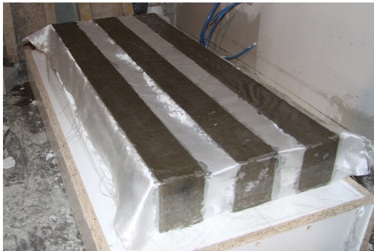
Figure D.4: The medium sized prismatic specimens coated with epoxy resin and one layer of glass fabric.
