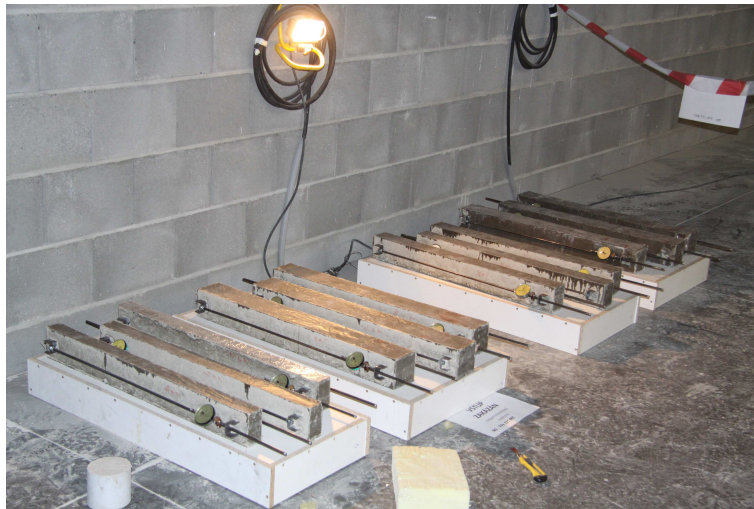
Figure D.7: Instrumented prismatic specimens, zero readings are taken (December 5 th ).
