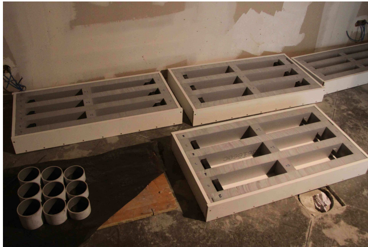
Figure D.1: Prepared mold for the four sets of prismatic specimens (different thicknesses) and three sets of cylinders (different heights).
