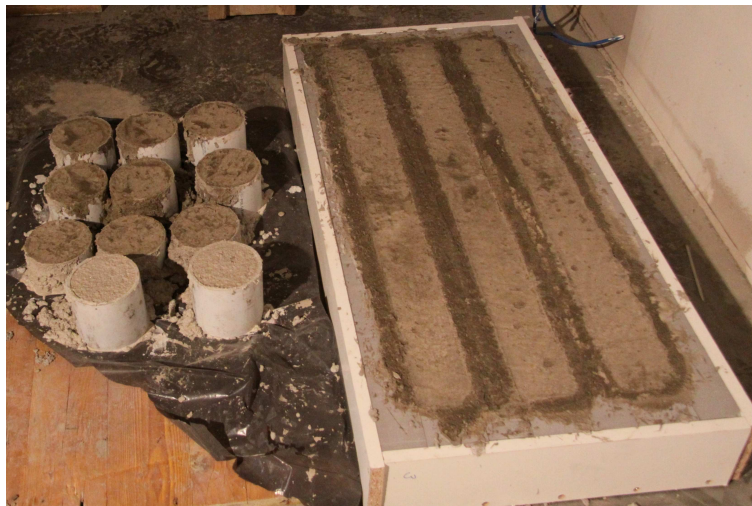
Figure D.2: Specimens at the age of three days, the prisms are just before demolding. Before this picture was taken, all specimens were covered with plastic foil to reduce evaporation.
