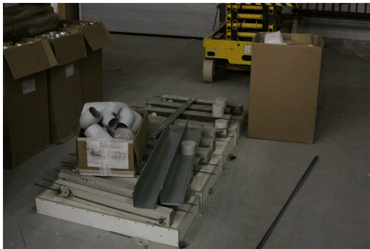
Figure D.8: Garbage placed on the top of the specimens, some of the gages shifted or destroyed. A yellow truck is parked just few centimeters next to the marks for the precise surveying (February 2014).
