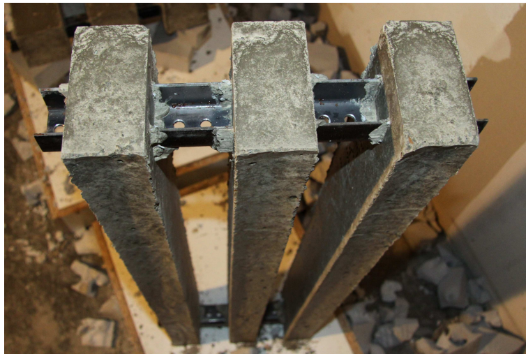
Figure D.3: Prismatic specimens just after demolding. The circular steel bars attached to the gages pass through the holes in the U-profile which in this picture holds the specimens together.
