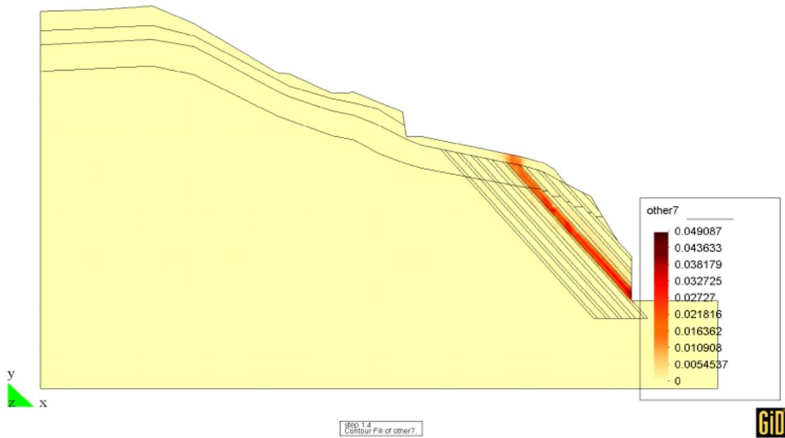
Figure 4.16: Segment of pier No. 10 (load combination 2, reached load factor  $\lambda_f = 1.4$ ) : Plastic zones - values of consistency parameter
