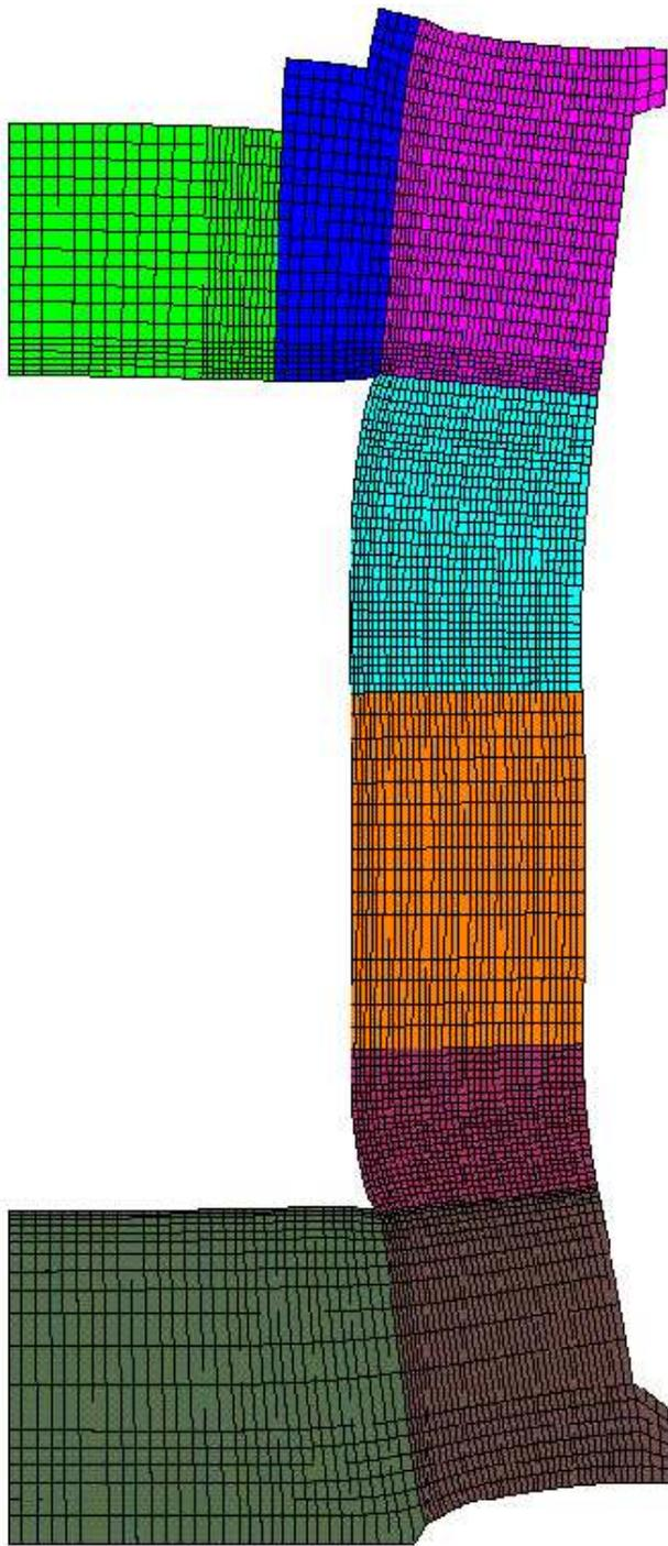
Figure 5: Deformed shape of the vessel caused by prestress.
