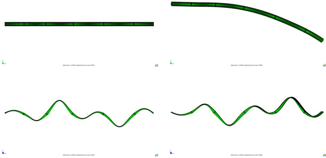
Figure 7: 7th eigenmode.
