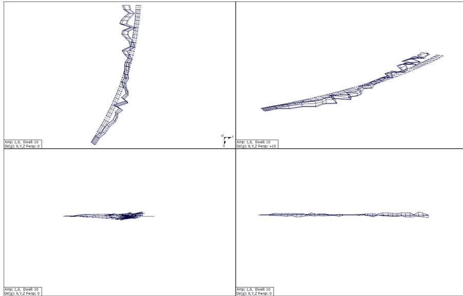
Figure 12: 2nd eigenmode.
