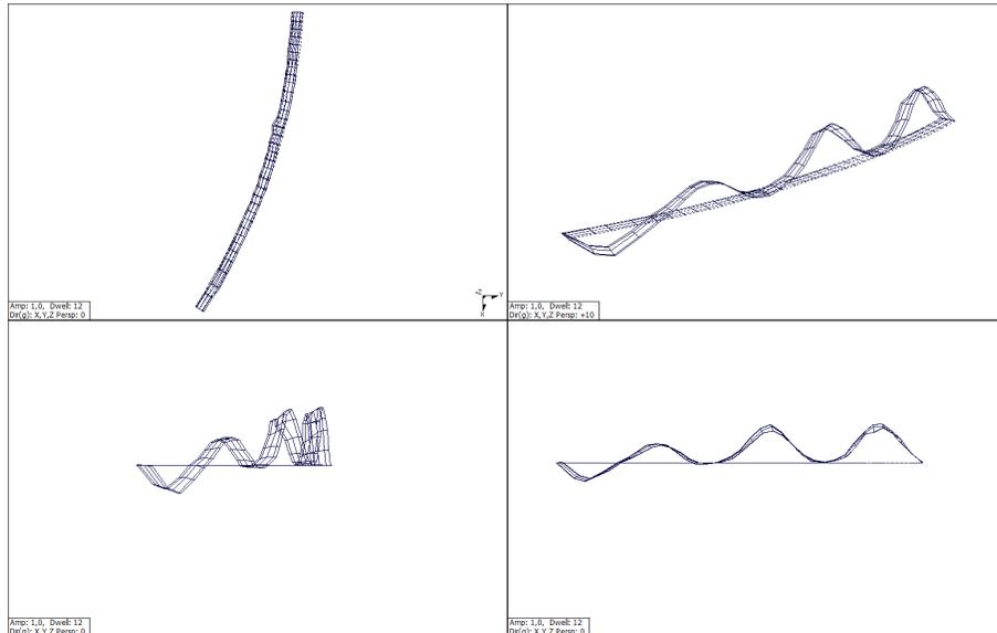
Figure 17: 9th eigenmode.
