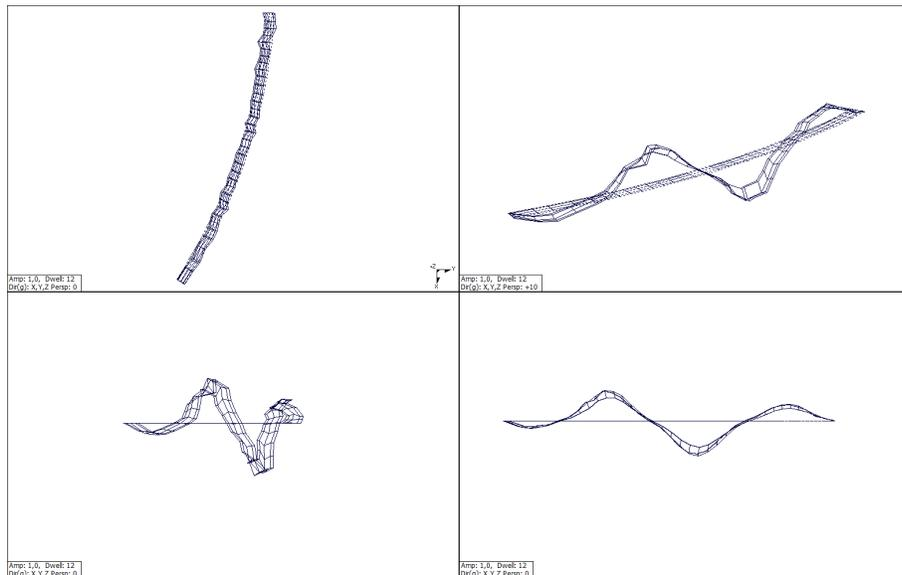
Figure 14: 4th eigenmode.
