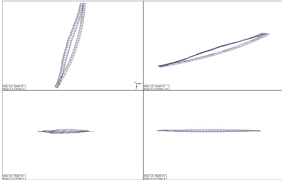
Figure 11: 1st eigenmode.
