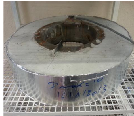
Fig. 1. Setup of the ring test (Courtesy of E. Rozière) [18].
