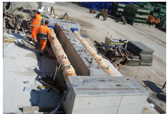
Fig. 16. A validated massive RG8 beam with restrained shrinkage (image from the Cheops database).
