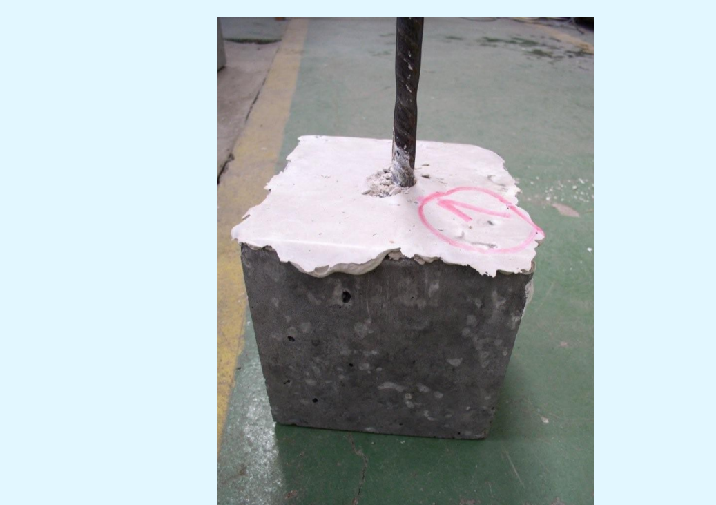
Pull-out test on the fly ash-based concrete.
