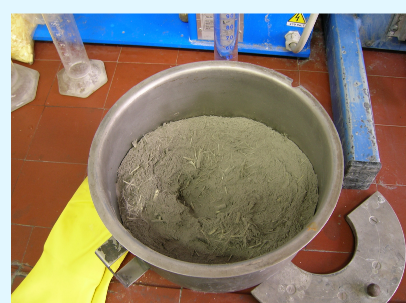
Fly ash with PP fibers before the addition of an activator and aggregates.
