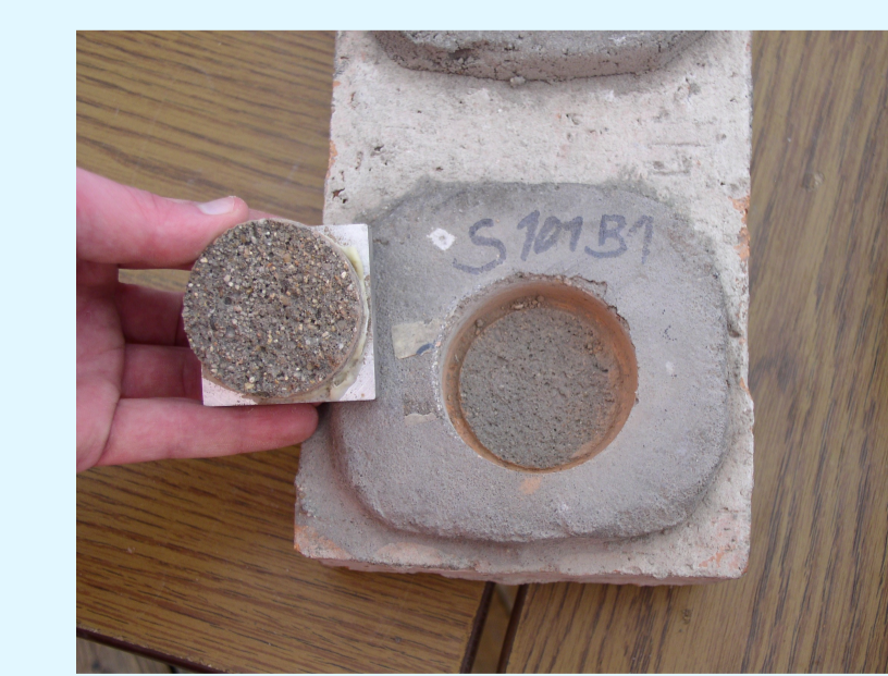
Tension tests of adhesive screed on the ordinary concrete.
