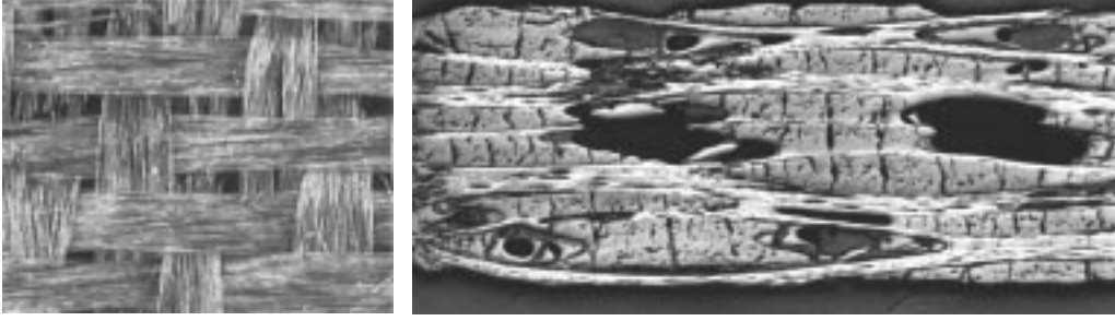
Fig. 1. An example of textile composite micrograph. Courtesy of B. Kořková, Technical University of Liberec
