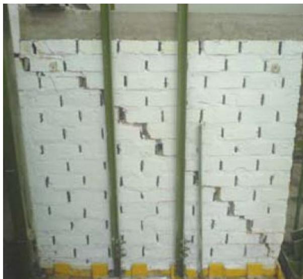
*Fig. 5.8: Crack pattern of experimental shear wall [29]*
