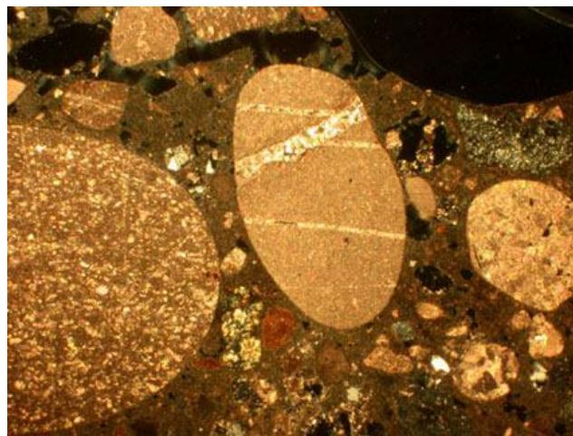
Fig. 1.2: Limestone pebbles as aggregates in non-hydraulic mortar [10]
