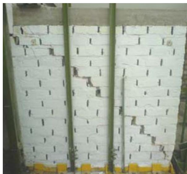
Fig. 5.8: Crack pattern of experimental shear wall [29]
