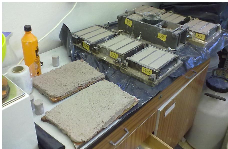
*Fig. 5.2: Samples of cocciopesto mortar in laboratory*
